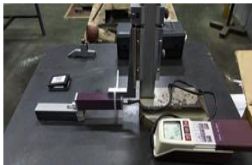
Gambar 3. Alat Uji Kekasaran Surface Roughness Tester seri SJ. 201P
